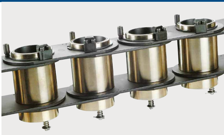
ATC magazine chain 340 with nickel-plated pots to house tools
